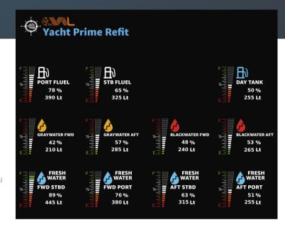
Embedded Color Display: 7", 10", or 19" (optional) with touch interface. Clear alarm visualization and quick controls.
